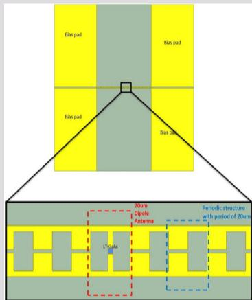
Excited by 100fs optical pulses with 15mW average power the T-Era-20D40P-800-air THz-PCAs generate 14nA peak THz photocurrent with more than 60dB THz power spectrum dynamic range.
