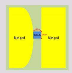
Excited by 100fs optical pulses with 20mW average power the T-Era-100A-1550-air THz-PCAs generate 250pA peak terahertz photocurrent with more than 50dB THz power spectrum dynamic range.
