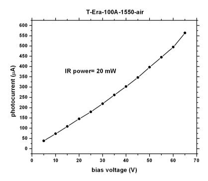
Figure 1. Photocurrent versus applied bias voltage across the T-Era-100A-1550-air THz-PCA.
