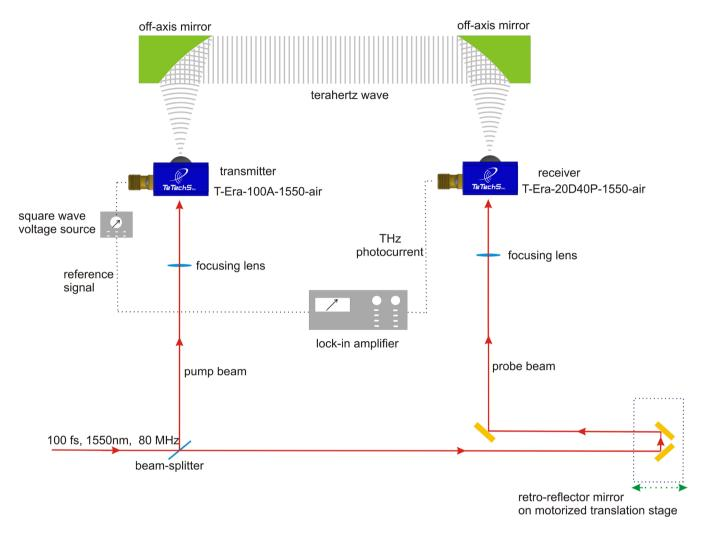
Figure 2. A terahertz response measurement setup for T-Era-100A-1550-air THz-PCA.
