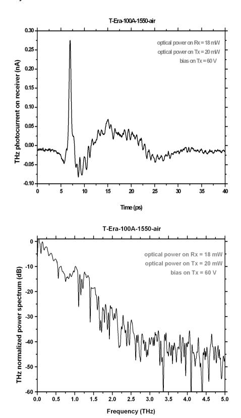
Figure 3. Typical THz pulse and its corresponding normalized power spectrum generated by a T-Era-100A-1550-air transmitter module and detected by a T-Era-20D40P-1550-air receiver module.
