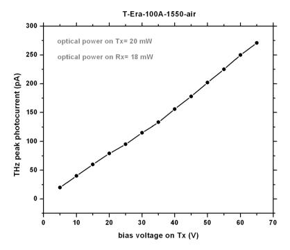
Figure 4. Terahertz peak photocurrent on T-Era-20D40P-1550-air receiver versus bias voltage over the transmitter T-Era-100A-1550-air.
