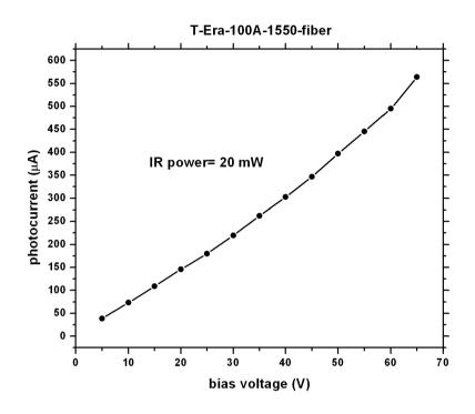
Figure 1. Photocurrent versus applied bias voltage across the T-Era-100A-1550-fiber THz-PCA.
