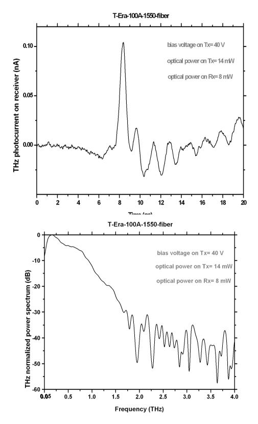
Figure 3. Typical THz pulse and its corresponding power spectrum generated by a T-Era-100A-1550-fiber transmitter module and detected by a T-Era-20D40P-1550-fiber receiver module.
