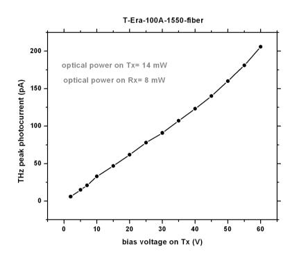
Figure 5. Terahertz peak photocurrent versus bias voltage on the T-Era-20D40P-1550-fiber receiver versus bias voltage on the T-Era-100A-1550-fiber transmitter.
