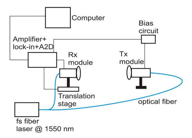
Figure 2. A terahertz response measurement setup for T-Era-100A-1550-fiber THz-PCA.
