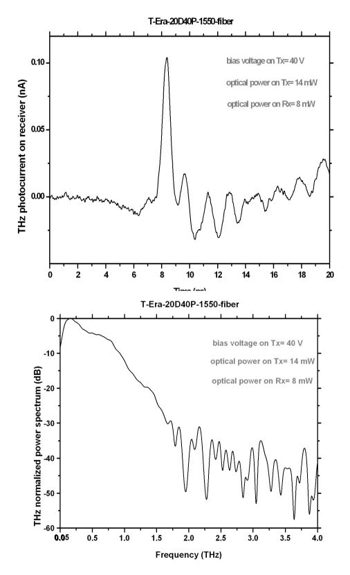
Figure 4. Typical THz pulse and its corresponding power spectrum generated by a T-Era-100A-1550-fiber transmitter module and detected by a T-Era-20D40P-1550-fiber receiver module.
