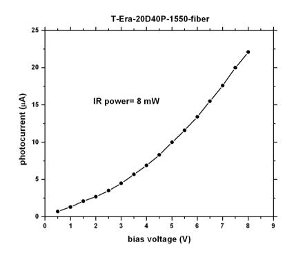
Figure 2. Photocurrent versus applied bias voltage across the T-Era-20D40P-1550-fiber THz-PCA.
