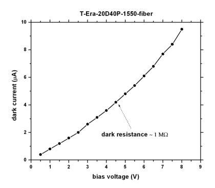
Figure 1. Dark current versus applied bias voltage across the T-Era-20D40P-1550-fiber THz-PCA.
