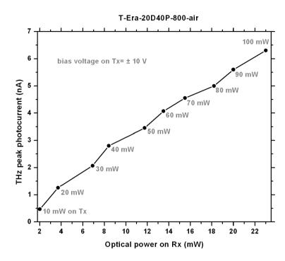
Figure 6. Terahertz peak photocurrent versus average optical power over the T-Era-20D40P-800-air THz-PCA. The average optical power on the transmitter module for each measurement point is shown on the graph.
