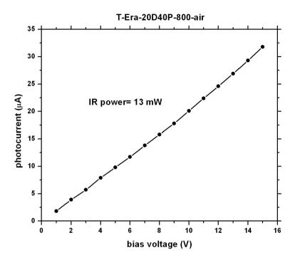
Figure 2. Photocurrent versus applied bias voltage across the T-Era-20D40P-800-air THz-PCA.
