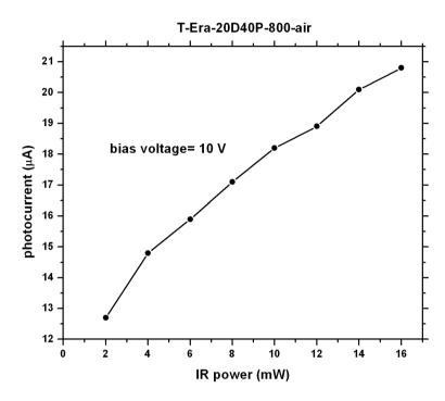
Figure 3. Photocurrent versus average optical power over the T-Era-20D40P-800-air THz-PCA.
