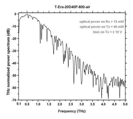
Figure 5. Typical THz pulse and its corresponding normalized power spectrum generated by a T-Era-100A-800-air transmitter module and detected by a T-Era-20D40P-800-air receiver module.
