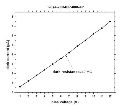
Figure 1. Dark current versus applied bias voltage across the T-Era-20D40P-800-air THz-PCA.
