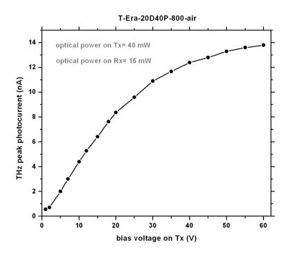
Figure 7. Terahertz peak photocurrent on T-Era-20D40P-800-air receiver versus bias voltage over the transmitter T-Era-100A-800-air.
