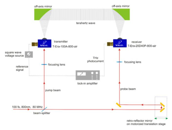
Figure 4. A terahertz response measurement setup for T-Era-20D40P-800-air THz-PCA.
