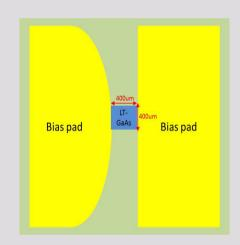
Excited by 100fs optical pulses with 50mW average power the T-Era-400A-800-air THz-PCAs generate 23 nA peak terahertz photocurrent with more than 50dB THz power spectrum dynamic range.
