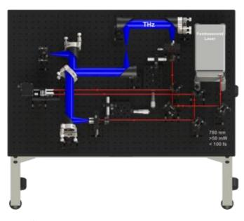
Optical and terahertz path schematic of the kit
