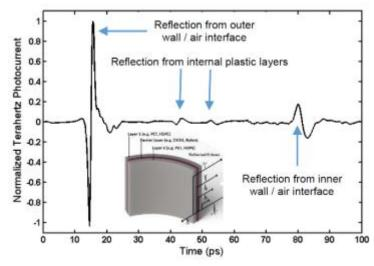
Example of a reflection terahertz measurement obtained with the measurement kit: Echo pulses off a multi-layer plastic
