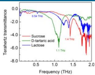
Example of a spectroscopy measurement of organic pow ders with the measurement kit
