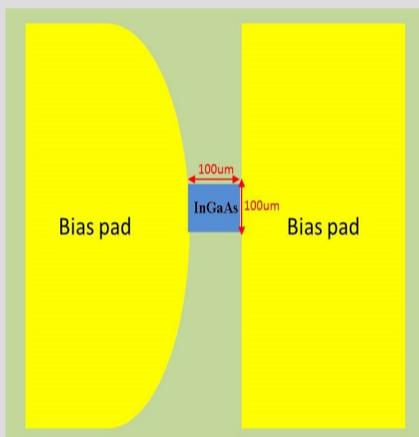
Excited by 100fs optical pulses with 14mW average power the T-Era-100A-1550-fiber THz-PCAs generate 200 pA peak terahertz photocurrent with more than 50dB THz power spectrum dynamic range.
