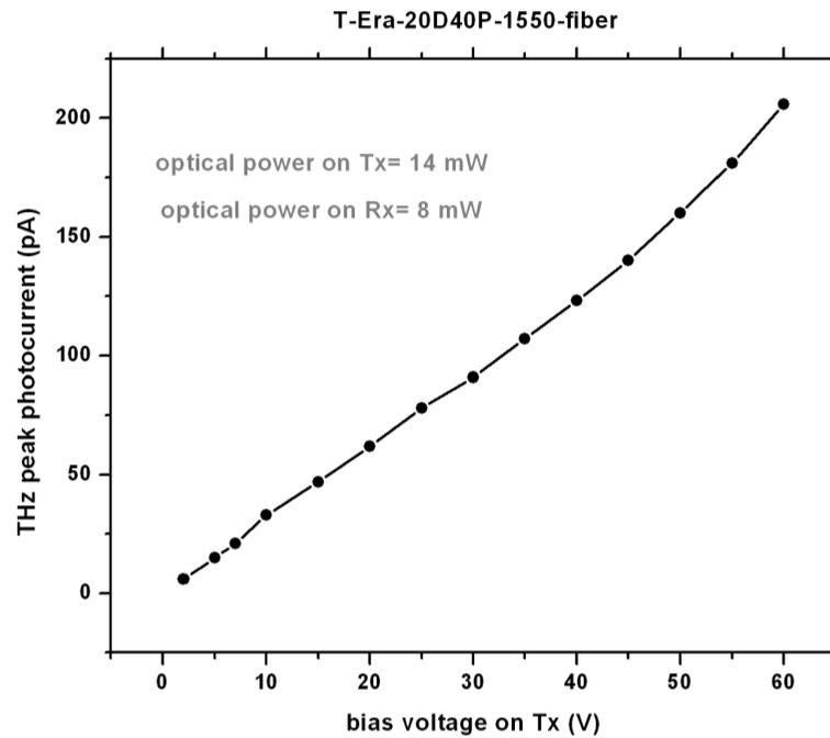
Figure 5. Terahertz peak photocurrent versus bias voltage on the T-Era-20D40P-1550-fiber receiver versus bias voltage on the T-Era-100A-1550-fiber transmitter.
