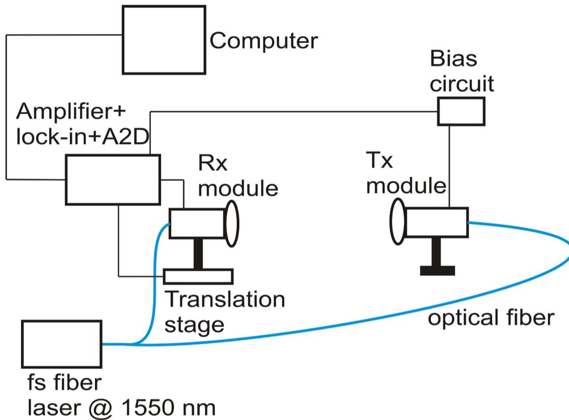
Figure 3. A terahertz response measurement setup for T-Era-20D40P-1550-fiber THz-PCA.
