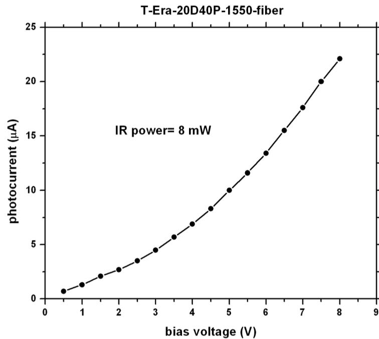
Figure 2. Photocurrent versus applied bias voltage across the T-Era-20D40P-1550-fiber THz-PCA.
