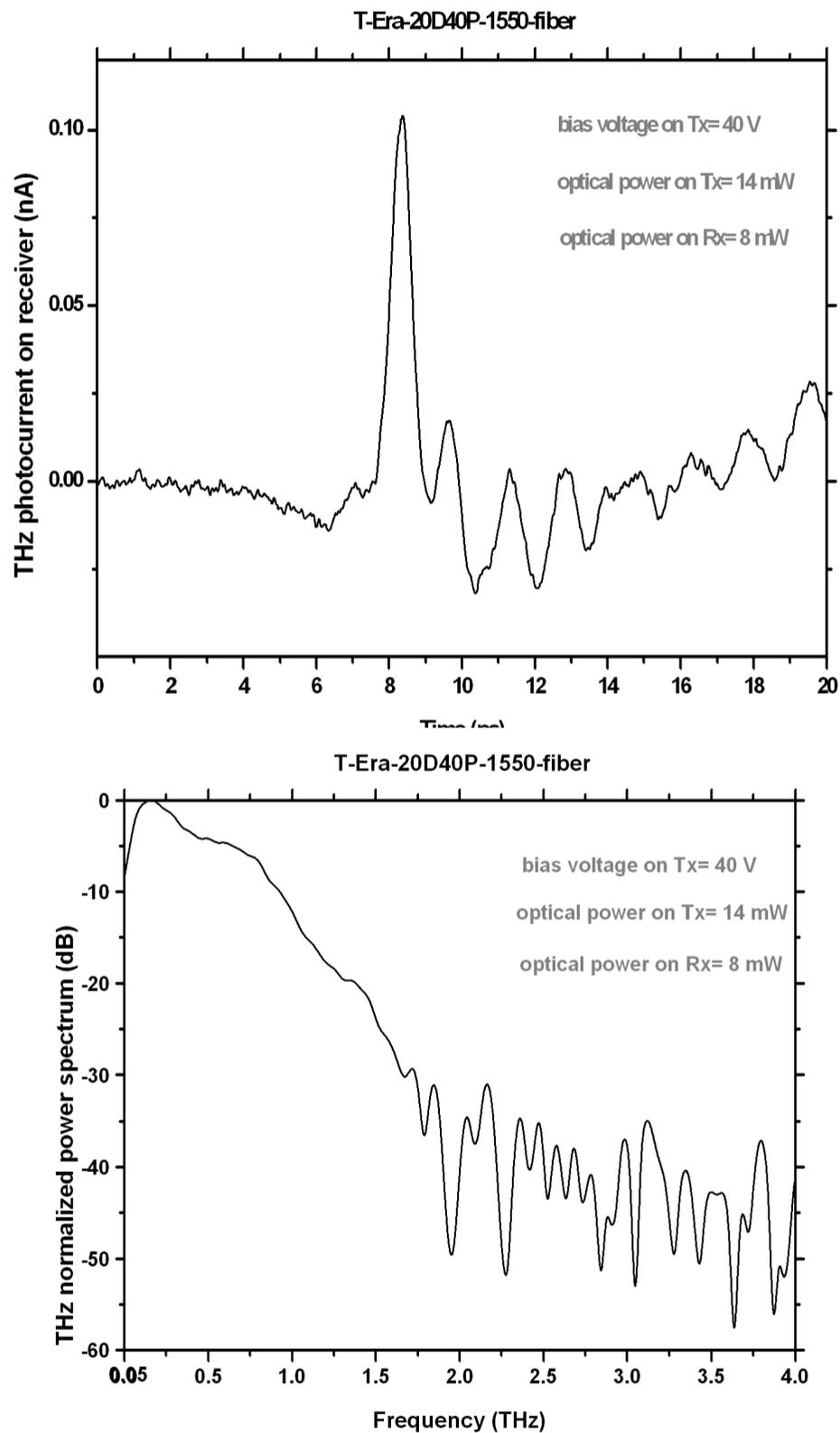
Figure 4. Typical THz pulse and its corresponding power spectrum generated by a T-Era-100A-1550-fiber transmitter module and detected by a T-Era-20D40P-1550-fiber receiver module.
