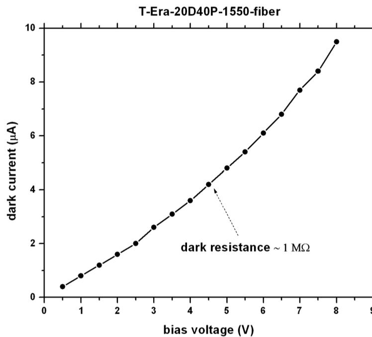
Figure 1. Dark current versus applied bias voltage across the T-Era-20D40P-1550-fiber THz-PCA.
