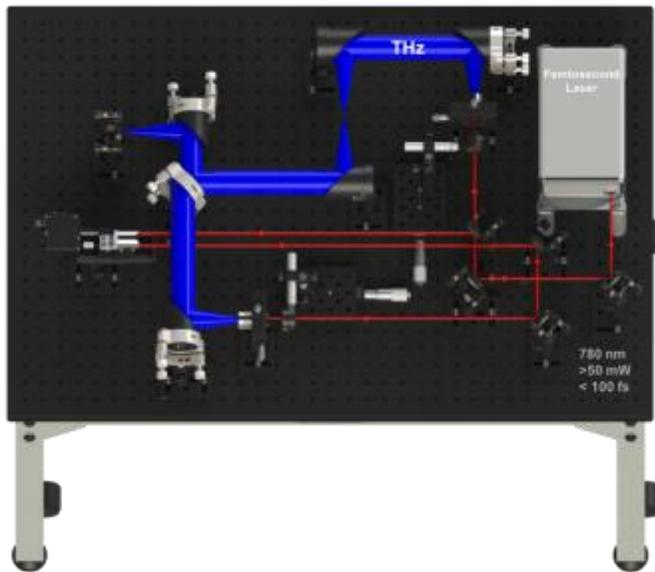
Optical and terahertz path schematic of the kit
