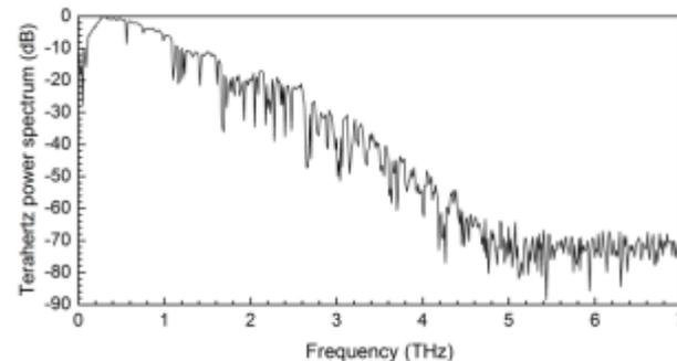
Example of a measured terahertz pulse and its corresponding power spectrum in the terahertz time-domain measurement kit shown in Figure 1 produced in 5 min.
